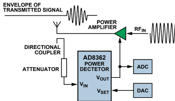
Figure 3. Power throughput detection.
