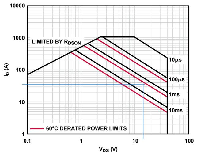
Figure 6. SOA plot including 62°C-derated power limits.
