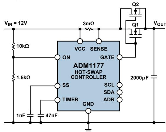
Figure 7. Completed reference design.
