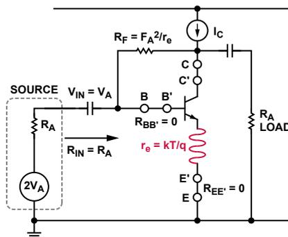
Figure 4. A rudimentary translinear LNA, illustrating the Fundamentals.
