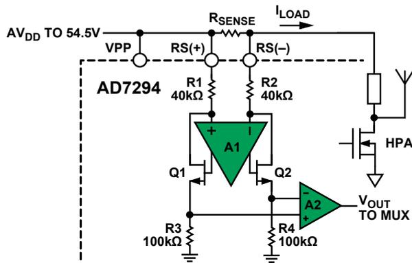
Figure 7. AD7294 high-side current-sense detail.
