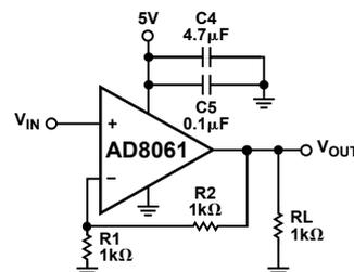
Figure 1. Noninverting op amp clock buffer.
