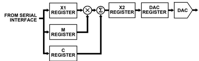
Figure 1. Single channel of AD5370 DAC.
