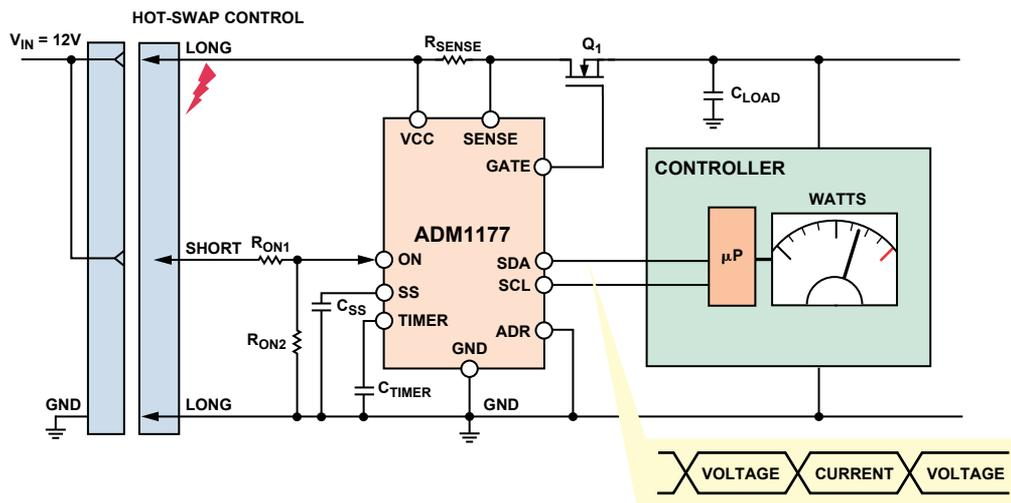
Figure 8. Hot swap with I<sup>2</sup>C digital power monitoring.
