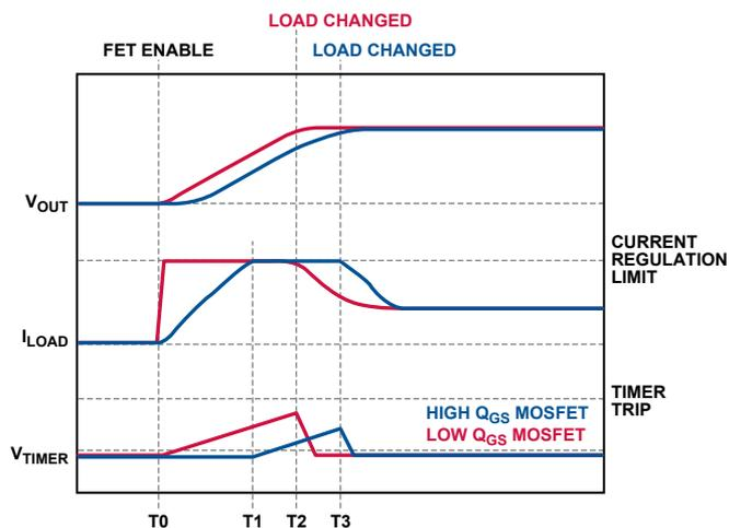
Figure 4. Effect of  $Q_{GS}$  on start-up profiles.
