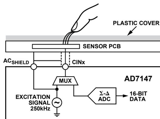
Figure 2. AC<sub>SHIELD</sub> eliminates capacitance between the sensors and the shield.
