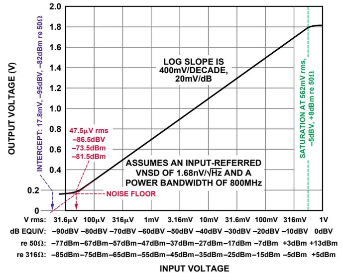
Figure 2. Log amp response to an input voltage, showing the lower bound on dynamic range, and the correspondence between alternative scales.
