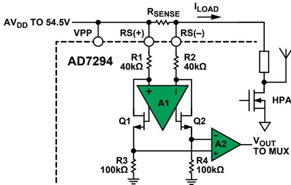
Figure 7. AD7294 high-side current-sense detail.
