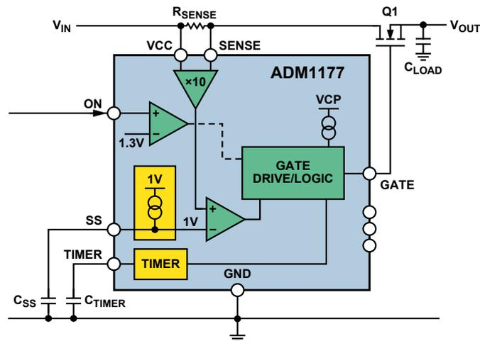
Figure 2. ADM1177 functional block diagram.
