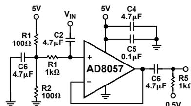
Figure 2. AC-coupled clock buffer (unity gain).
