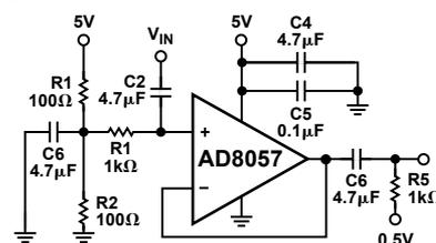
Figure 2. AC-coupled clock buffer (unity gain).
