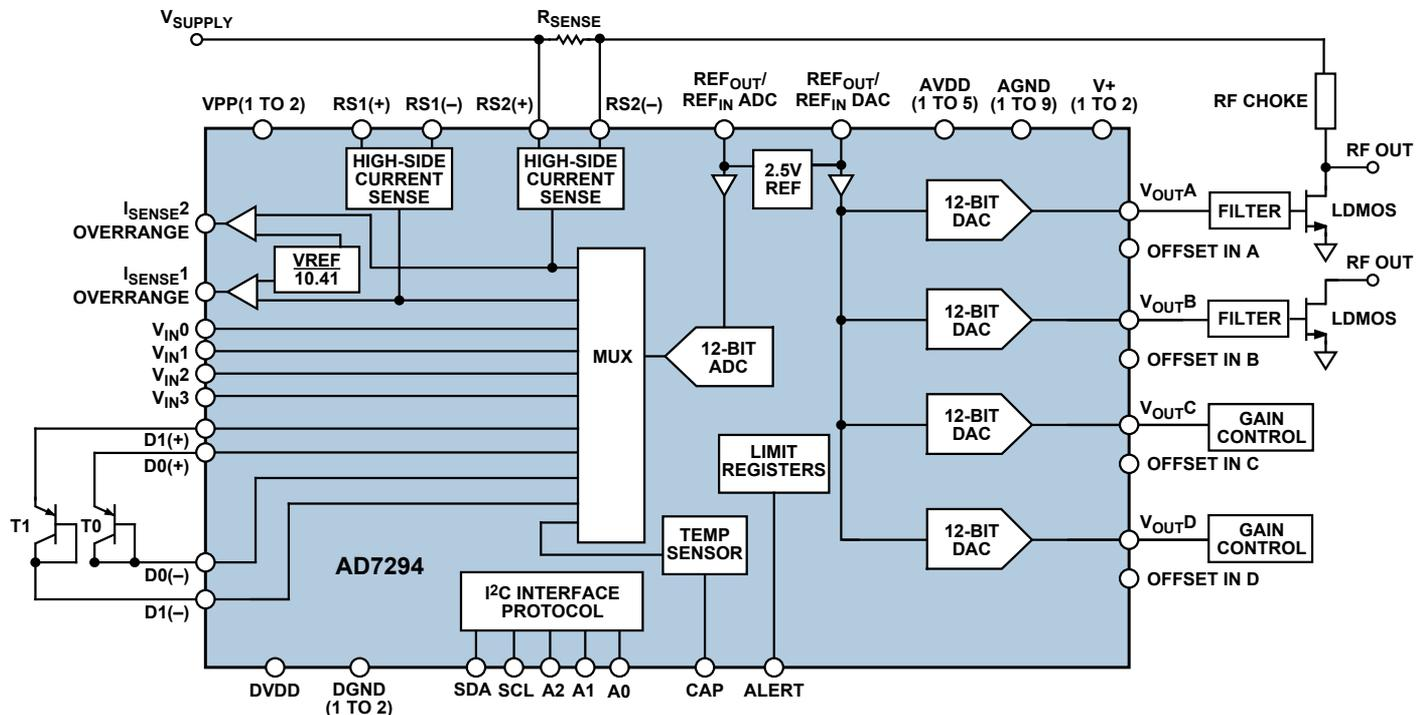
Figure 6. Integrated solution for monitoring and controlling PA stages.
