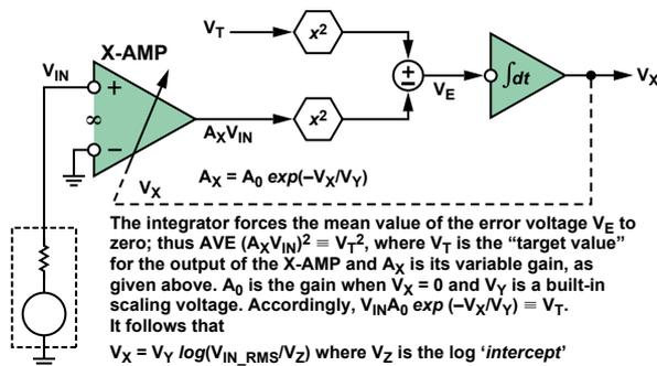
Figure 6. General structure of an AGC-style log amp.
