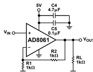
Figure 1. Noninverting op amp clock buffer.
