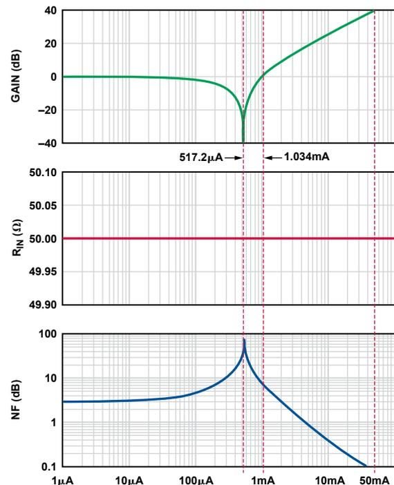
Figure 5. The peculiar behavior of the translinear low-noise amplifier.
