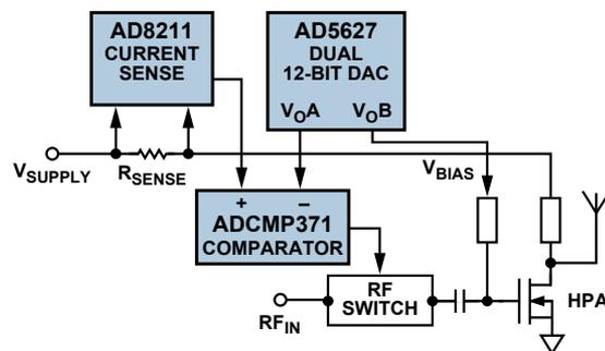
Figure 4. Control-loop protection using an analog comparator.
