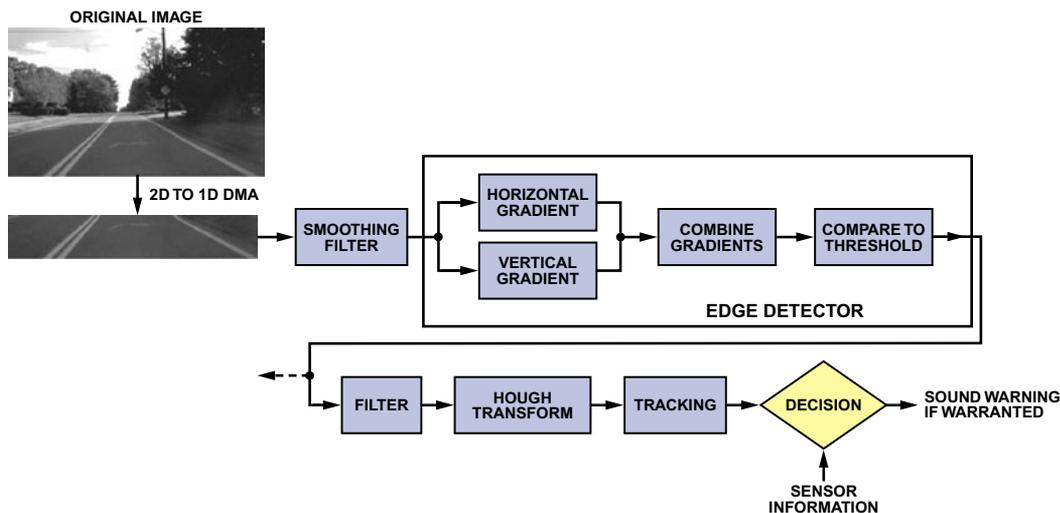
Figure 3. Algorithm flow, showing results of intermediate image-processing steps.
