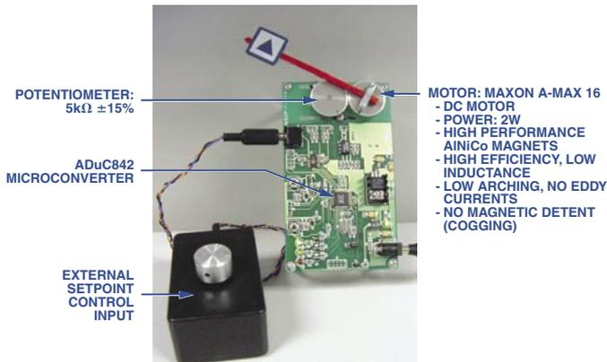
Figure 5. Sample motor control system using discrete components.
