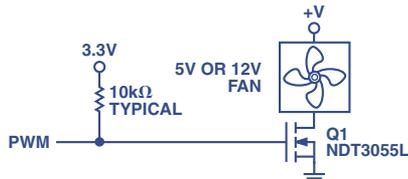
Figure 5. A low-frequency PWM fan-drive circuit.
