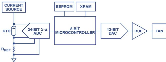
Figure 2. Example of a PID controller for a temperature-controlled ventilation system using discrete components.
