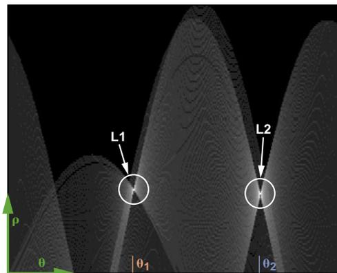
Figure 8c. The Hough transform of the image in Figure 8a. The range for  $\theta$  is  $[0, 2\pi]$ , and the range for  $\rho$  is one-half the diagonal of the input image in Figure 8a. The two bright regions correspond to local maxima, which can be used to reconstruct the two lines in Figure 8a.
