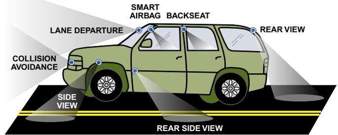
Figure 1. Basic camera-placement regions for automotive safety applications.
