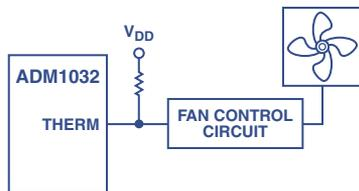
Figure 3. Example of an on/off control circuit.
