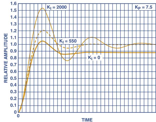
Figure 7. Proportional-integral (P-I) control for three settings of the integral term. Note the offset from 1.0 for  $K_I = 0$ , the lightly damped oscillatory tendency for  $K_I = 2000$ , with oscillations almost eliminated at  $K_I = 550$ .
