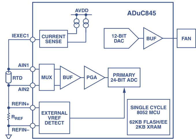
Figure 3. System-on-a-chip implementation.
