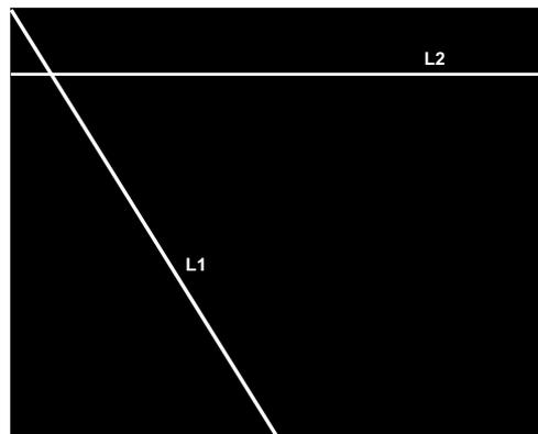
Figure 8a. The output of an edge detector is a binary image like this one, which can be visually inspected by a human observer to show lines. A Hough Transform allows localization of these two lines.
