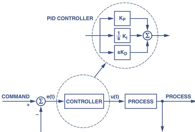
Figure 1. Control loop employing a PID control function.
