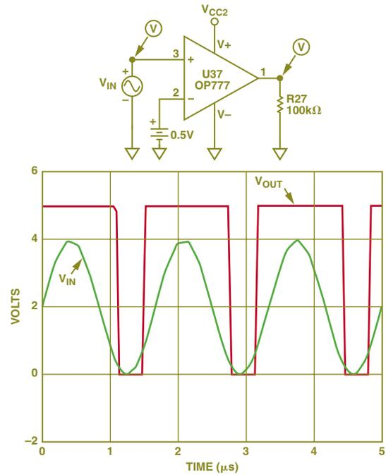
Figure 3. Response of an OP777 amplifier to a  $\pm 2$ -V, 1-kHz signal, biased by +2V, and compared with a +0.5-V dc level. Note that there is no phase inversion for this large swing. However, the gain is quite low at a common-mode level of +0.5 V from the negative rail, as can be seen by the approximately 0.3-V overdrive that is needed.
