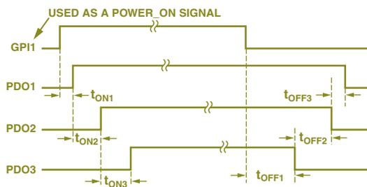
Figure 4. Controlled power on/off sequence using the ADM1060. Providing the same seven supplies outlined in the discrete design of Figure 1, a sequence could be implemented using a single ADM1060 as shown in Figure 3.
