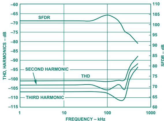
Figure 4. THD, second and third harmonics, and SFDR vs. frequency. SFDR scale is at right.
