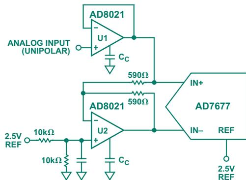
Figure 5. A single-ended to differential-input ADC driver circuit.
