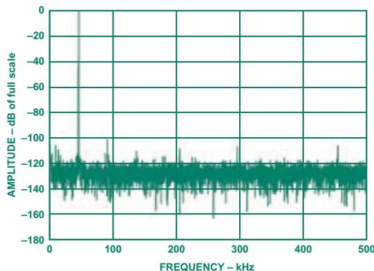
Figure 3. FFT plot of AD7671/AD8021 combination.
