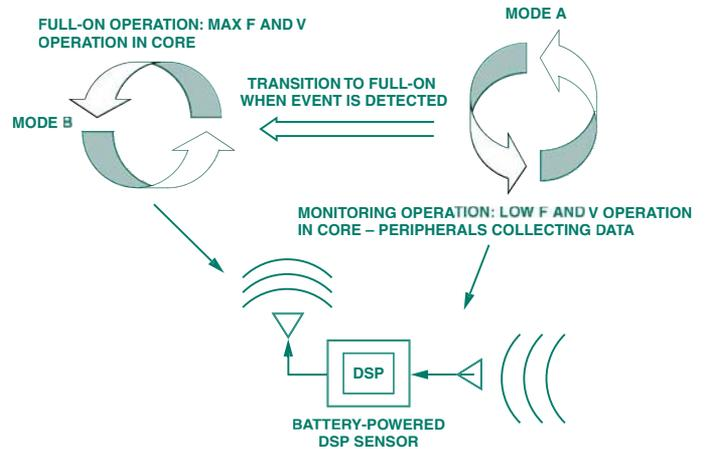
Figure 4. Sample DSP application with different operating modes.
