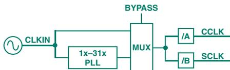
Figure 3. Functional block diagram of ADSP-21532 clock-generation unit.
