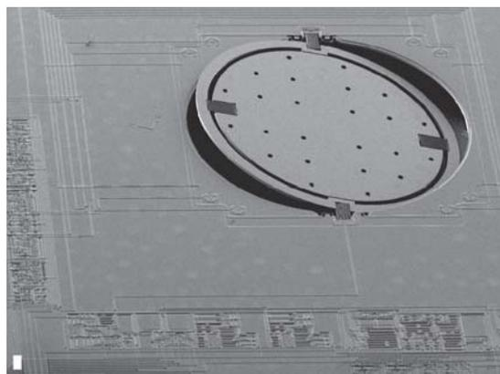
Figure 4. SEM of fabricated mirror with integrated circuitry.
