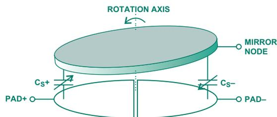
Figure 1. Capacitive bridge established by mirror structure.
