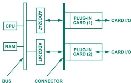
Figure 11. Using the ADG3247 in a hot-plug application.
