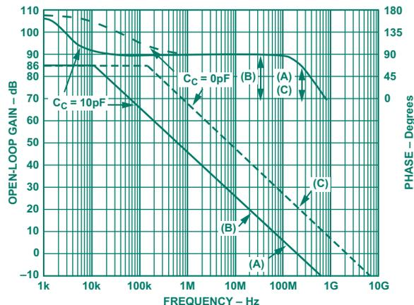
Figure 8. AD8021 open-loop gain and phase vs. frequency.
