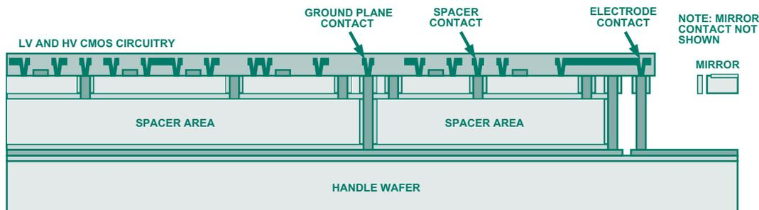
Figure 3. Analog Devices optical iMEMS process—optical mirror fabrication with integrated circuitry.
