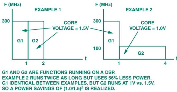
Figure 2. Power dissipation vs. frequency and time.
