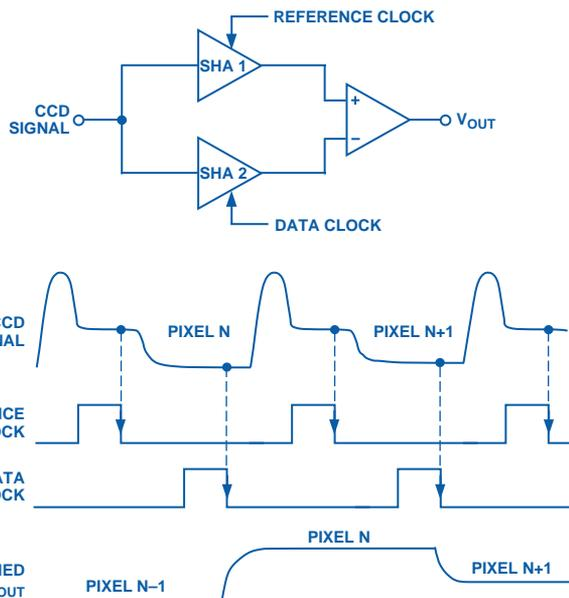
Figure 2. Correlated double sampling. SHA1 samples the reference level, SHA2 the data level. The difference amplifier subtracts the samples, for a measure of the light intensity, reducing common-mode noise.
