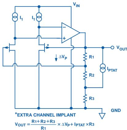
Figure 1. Simplified schematic diagram of ADR29x reference.
