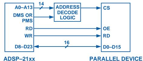
Figure 3. Parallel I/O interfacing for a DSP.
