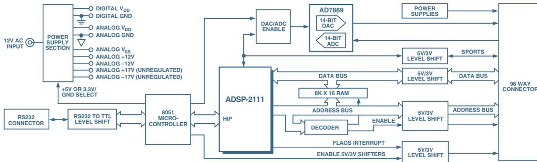
Figure 2. Block diagram of the Evaluation-Control Board.
