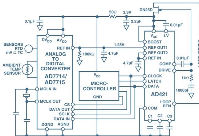
Figure 4. Details of a Smart Transmitter.
