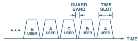
Figure 1. Illustration of time multiplexing, showing guard bands.
