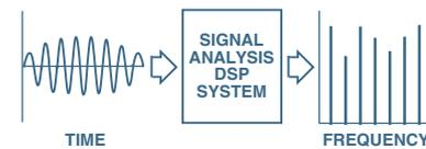
Figure 7. Example of batch processing of a block of data.
