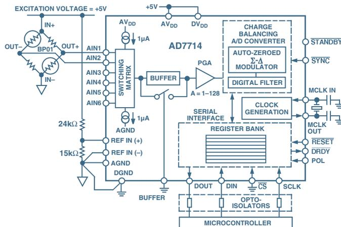
Figure 5. Interfacing a transducer interface to AD7714 ADC.
