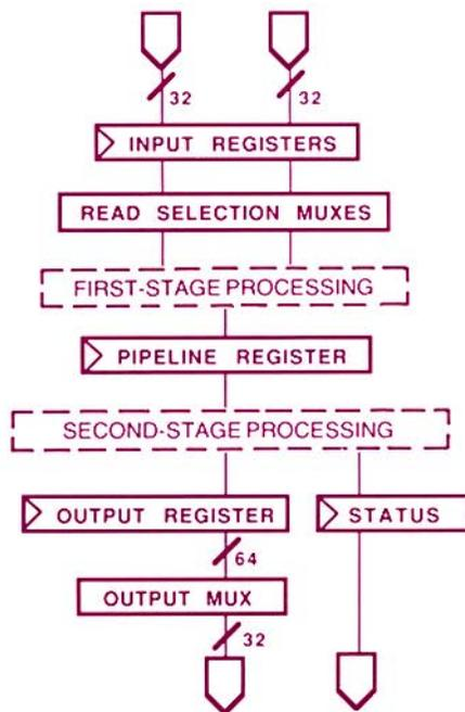
Figure 1. Generic architecture of ADSP-32XX number-crunchers.
