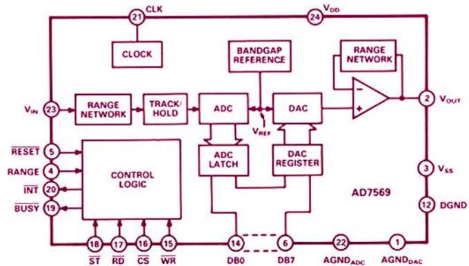
Figure 1. Functional block diagram of the AD7569.
