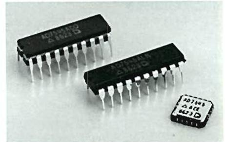
has  $\pm$ 1-LSB maximum gain error when powered from a single +5-volt supply; this provides high precision in 5-volt operation (with both TTL and CMOS compatibility).
