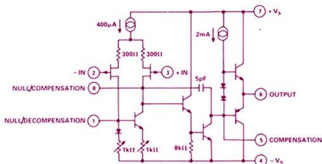
Figure 1. The simplified schematic of the AD744 shows the relatively simple two-stage architecture.
