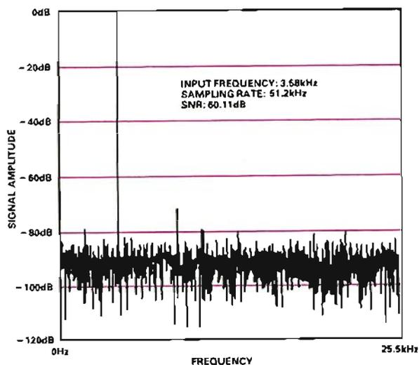
Figure 2. FFT Spectral Response of the AD7579/AD7580.
