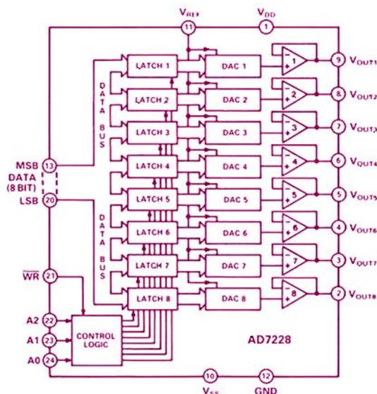
Figure 1. The AD7228 has 8 DACs on a CMOS chip.
