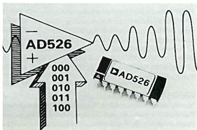
( $\Delta V_{OUT} = \pm 10$  V) of from 4 to 7  $\mu$ s, depending on the gain setting. Minimum slew rate is 4 V/ $\mu$ s for gains of 1, 2, and 4—increasing to 18 V/ $\mu$ s for gains of 8 and 16; and full-power bandwidth at gain of 16 is 350 kHz.
