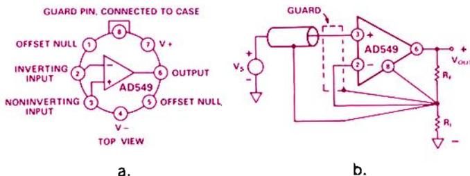
Figure 2. Guard pin for reduced leakage and current noise. a. Connection diagram, showing guard pin. b. Non-inverting amplifier with guard.
