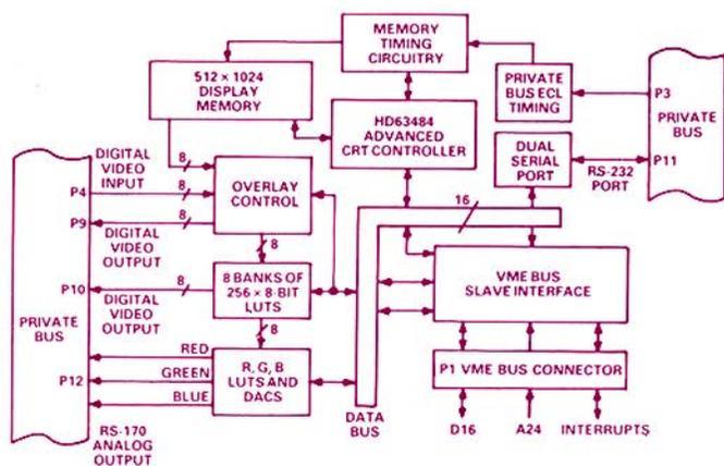
Figure 2. The RTI-681-HS block diagram shows the bus interfaces, dual serial port, and RGB analog output.
