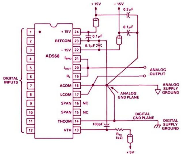
Figure 2. Basic connections for  $\pm 1.024\text{-volt}$  full-scale output.
