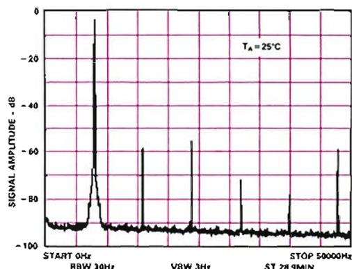
Figure 2. The DAC Output Spectrum for 8-kHz output, using a swept filter analyzer with 3-Hz filter bandwidth.
