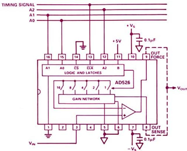
Figure 2. Operation in latched mode.
