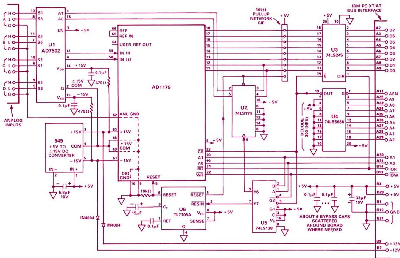
Figure 4. Interfacing to the IBM PC/XT/AT.
