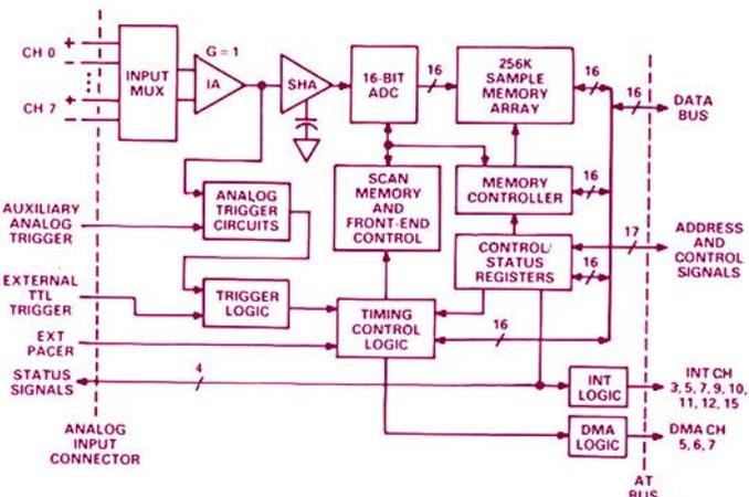
Figure 1. Block diagram of RTI-850 shows 8-channel differential input multiplexer and 16-bit ADC.
