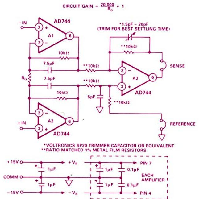
Figure 5. Use of AD744 as a high performance instrumentation amplifier, with gains from 1 to 1,000 set by resistance  $R_G$ .
