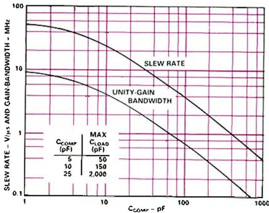
a. Effect of compensation capacitance on unity-gain bandwidth, slew rate, and ability of the AD744 to drive a capacitive load.
