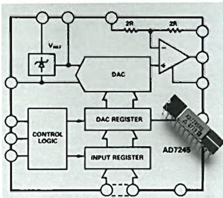
The AD7245\* and AD7248 are complete monolithic 12-bit CMOS d/a converters, housed in a 24-pin "skinny" DIP. The LC<sup>2</sup>MOS (linear-compatible CMOS) process makes it possible to include the DAC, output amplifier, voltage reference, control logic and double-buffer latches on a single compact chip.
