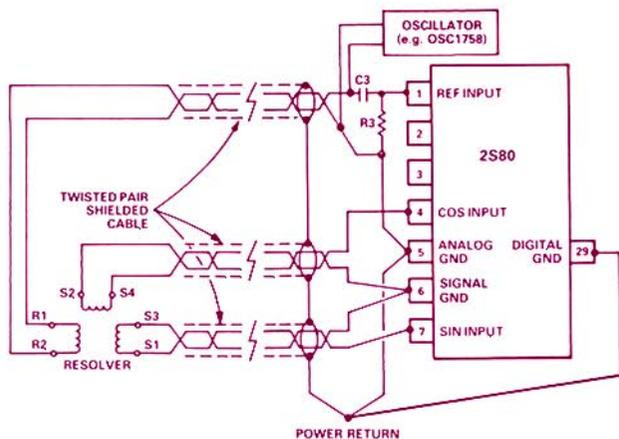
Figure 1. Resolver and resolver-to-digital converter.
