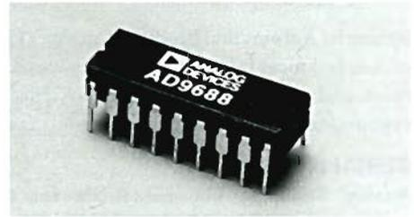
The AD9688\* is a 4-bit, high-speed analog-to-digital converter with ECL-compatible outputs. Fabricated in a high-performance bipolar process, it allows full Nyquist operation at up to 200-Msps encoding rates.
