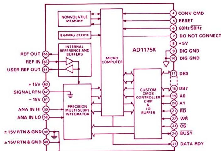
Figure 1. Block diagram and connections of the AD1175.
