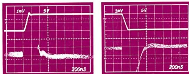
Figure 2. Typical settling time of AD744 as an inverter in response to 0 to +10-volt and 0 to -10-volt square waves (scales: 5 V/div for square wave, 1 mV/div for response, time = 200 ns/div).
