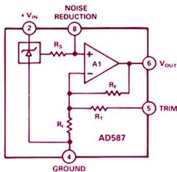
Figure 1. Functional block diagram of the AD587. The AD586 is similar but uses a voltage divider on the Zener output.
