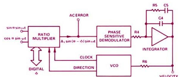
Figure 2. Functional diagram of the 2S80.
