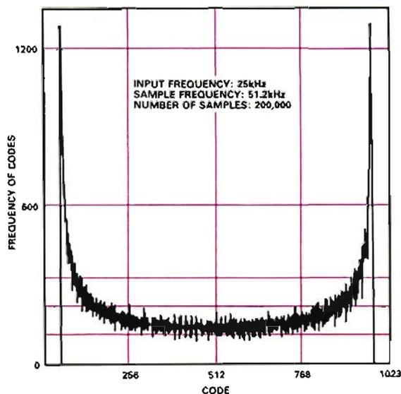
Figure 3. Histogram plot showing frequency of occurrence for each ADC output code.
