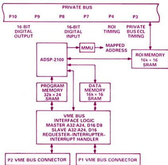
Figure 1. The RTI-680-HS block diagram shows the ADSP-2100 DSP microprocessor, region-of-interest memory, and private high-speed bus.
