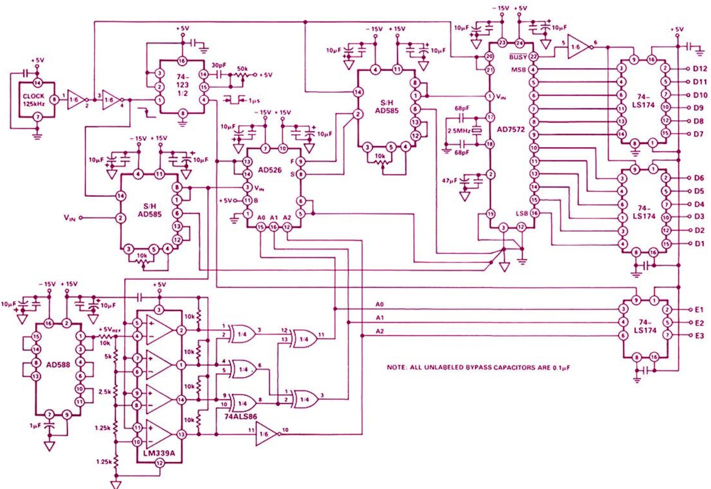
Figure 3. Floating-point a/d converter.
