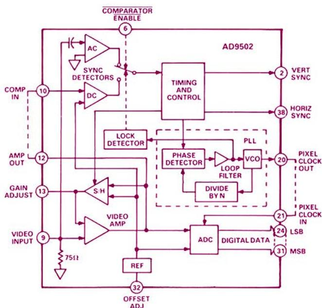
Figure 2. Functional block diagram of the AD9502.
