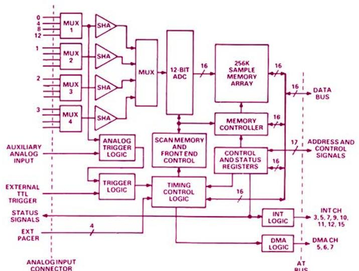
Figure 2. RTI-860 has 4 track-holds to ensure that data is immediately ready for the next conversion.
