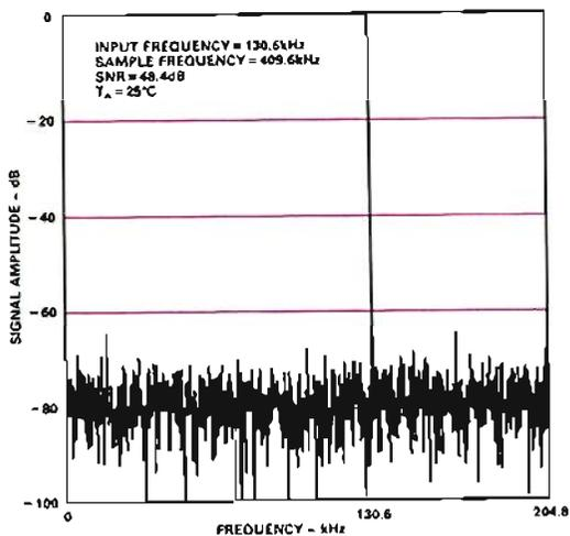
Figure 3. FFT plot of ADC performance, with input of 130.6 kHz, and sampling at 409.6 kHz.
