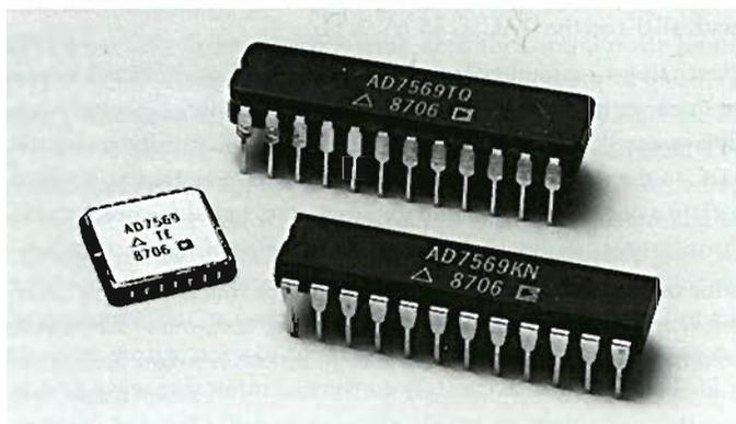
CMOS (<80mW maximum) and low supply-current requirements minimize heat problems in these designs. The price of this component is less than the cost of buying, assembling, and testing the individual functional elements—only \$6 in 100s.
