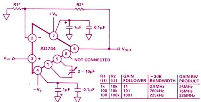
Figure 4. Extending the gain bandwidth product through the use of an external "decoupling" capacitor, for a noninverting configuration.
