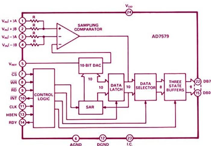
Figure 1. Block diagram of the AD7580. The AD7579 has the same functions, but the 10-bit-wide digital interface is replaced by a multiplexed 8-bit interface.
