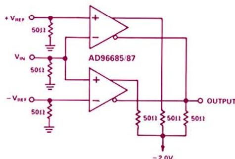
Figure 2. Basic connections for high-speed window comparator.
