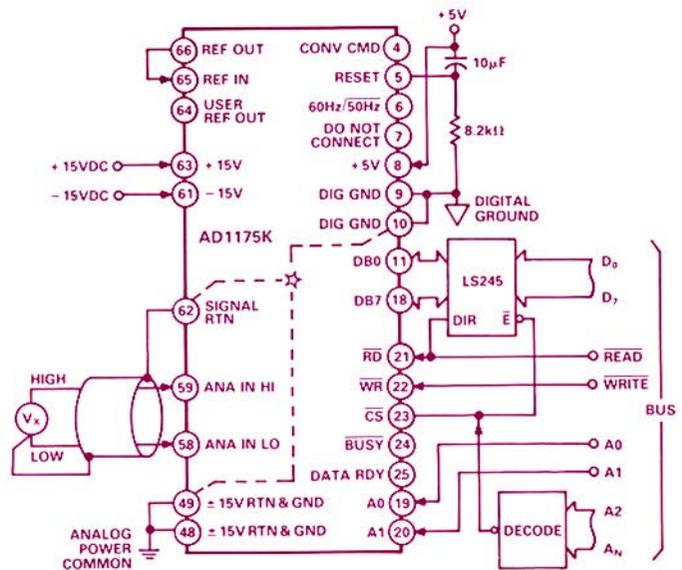
Figure 3. Interfacing to a bus—basic connection.
