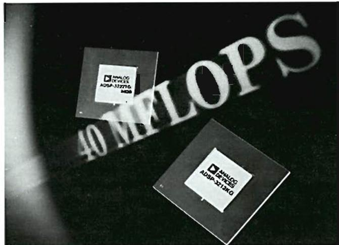
Both devices support 32-bit and 64-bit IEEE-754 floating-point operation, as well as 32-bit fixed-point twos-complement, unsigned magnitude, and mixed-mode arithmetic. Versions that support DEC formats F and G (the ADSP-3213 and ADSP-3223) are also available. Typical applications include high-performance digital signal-processing, engineering workstations, floating-point accelerators, array processors, mini-supercomputers, and RISC (reduced instruction-set computer) processors.
