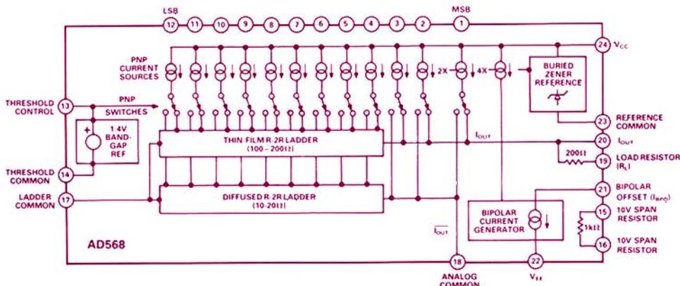
Figure 1. Block diagram of the AD568.
