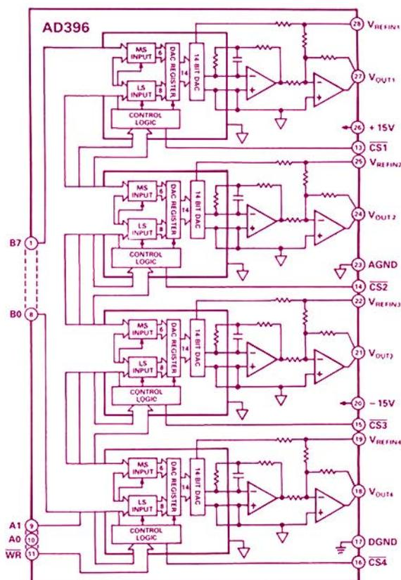
Figure 2. Block diagram of the AD396 quad DAC.
