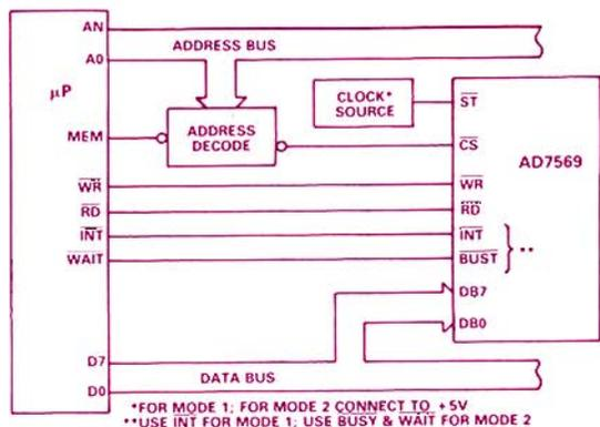
Figure 4. Connection between the AD7569 and microprocessor busses, for both periodic clock and read-cycle-initiated conversions.
