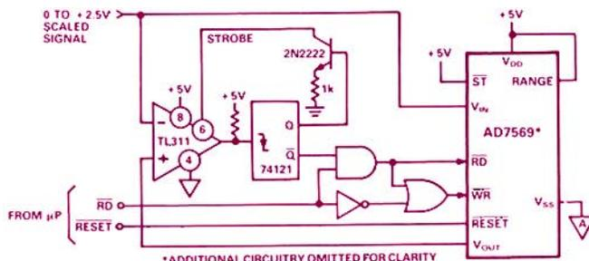
Figure 5. Peak-reading circuit uses the functions of the AD7569, requires no processor or software support, and has no droop.
