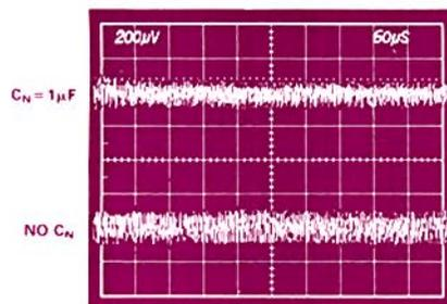
Figure 2. Effect of 1- $\mu\text{F}$  noise-reduction capacitor on broadband noise.
