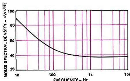
Figure 1. Input voltage-noise spectral density.
