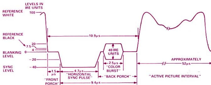
Figure 1. Annotated video signal shows key elements of horizontal timing and intensity standards.
